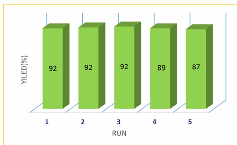
Fig. 1. Catalytic activity of Cu/C in five cycles for the synthesis of 1-substituted 1H-tetrazoles.
