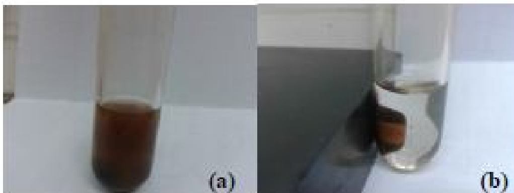
Fig. 7. a) Reaction mixture, b) Separation of Pd-Py- \gamma -Fe 2 O 3 by an external magnetic field.
