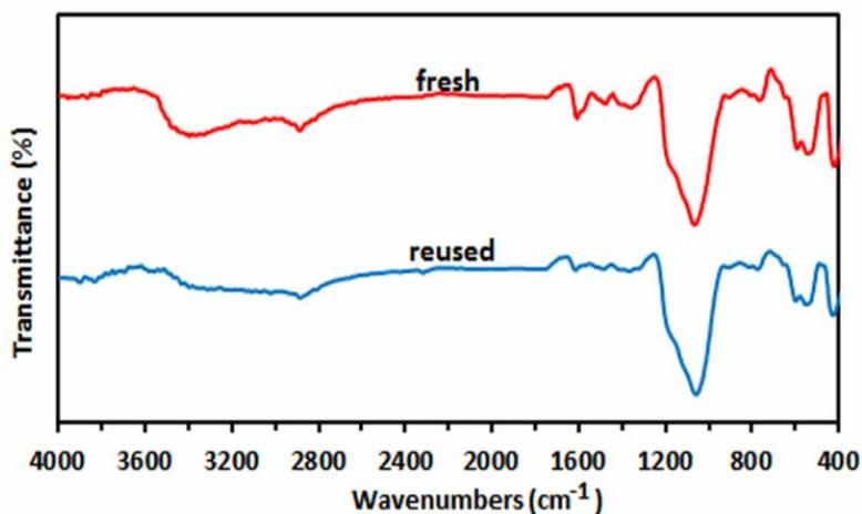
Fig. 9. The FT-IR spectra of the fresh catalyst and the six-times reused catalyst.
