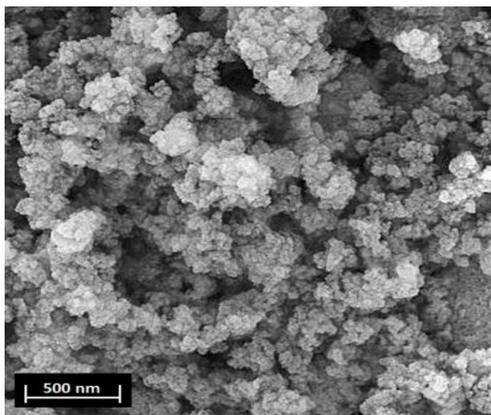
**Fig. 2.** The FE-SEM images of MNPs-TBAN nanoparticles.
