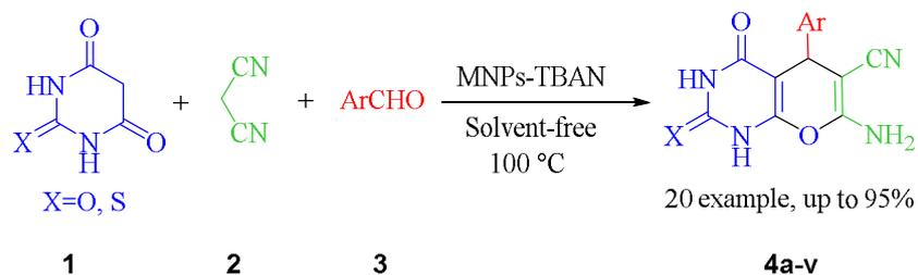
**Scheme 2.** Multicomponent synthesis of pyrano[2,3-*d*]pyrimidine using bis(4-(dimethylamino)anilino)triazine-grafted on silica-coated magnetite nanoparticles (MNPs-TBAN)
