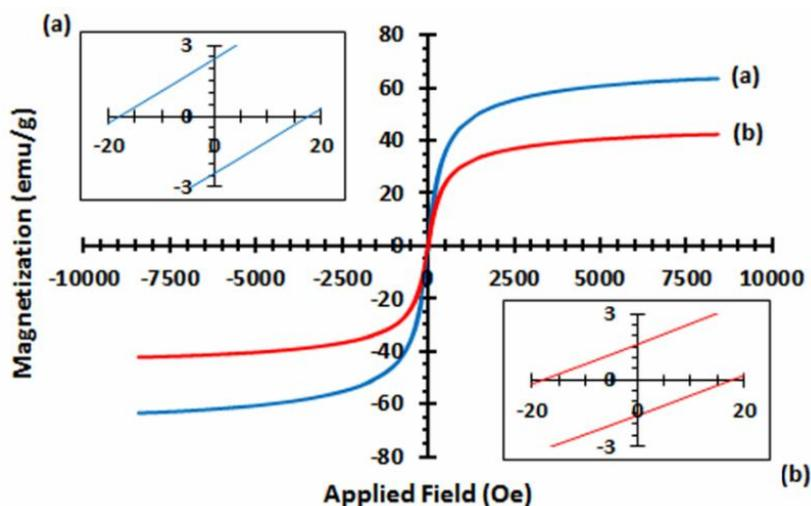
**Fig. 7.** The magnetic hysteresis loops of  $\text{Fe}_3\text{O}_4$  MNPs (a) and MNPs-TBAN (b). Left and right inset: the magnified zone from -20 to 20 Oe.
