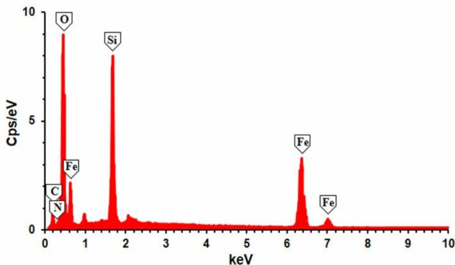
Fig. 3. The EDS spectrum of MNPs-TBAN nanoparticles.
