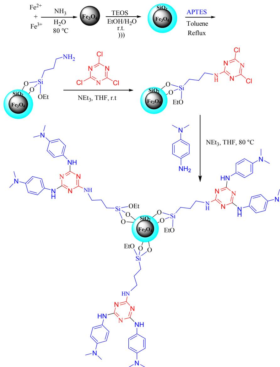
*Scheme 1.* Preparation of bis(4-(dimethylamino)anilino)triazine-grafted on silica-coated nano-Fe<sub>3</sub>O<sub>4</sub> particles (MNPs-TBAN)
