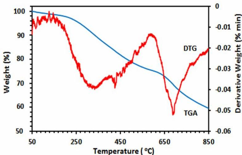
Fig. 6. The TGA and DTG curves for MNPs-TBAN nanoparticles.
