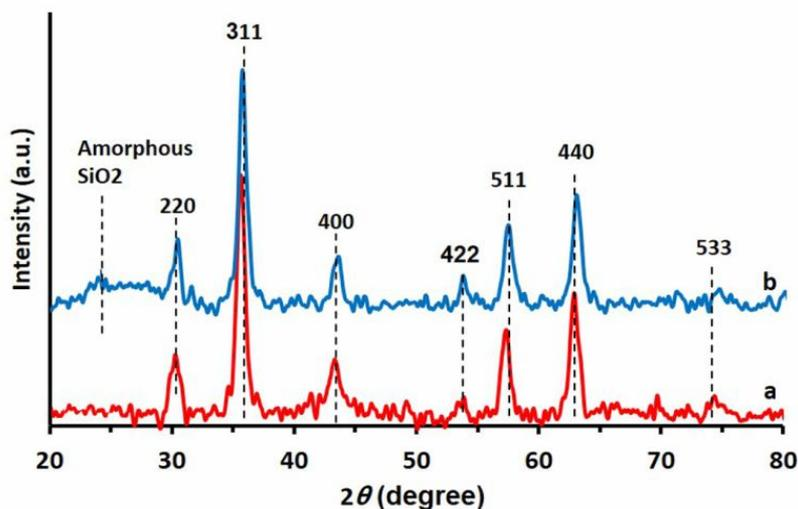
Fig. 5. The XRD patterns of (a)  $\text{Fe}_3\text{O}_4$  and (b) MNPs-TBAN.
