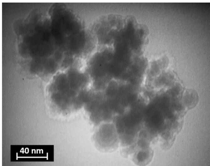
Fig. 4. The TEM image of MNPs-TBAN nanoparticles.
